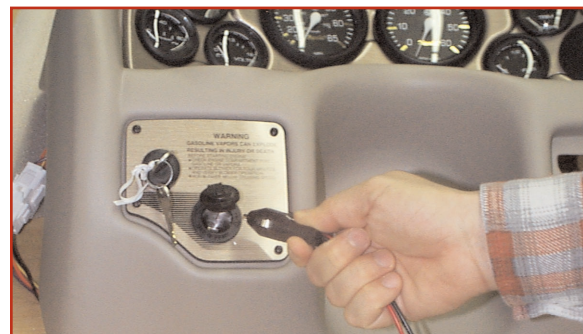
Figure 4 - Attaching the adapter cable's cigarette plug to the dashboard's 12V receptacle.
