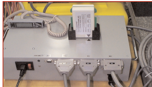
Figure 3 - Connecting the umbilical cables to the Application Interface Box
